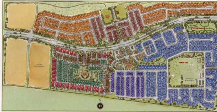
The Village of Five Parks in Arvada, Colo., mixes TND principles with those of conventional subdivisions. The front-loaded Haven homes (light blue) — on 60x100-foot lots and ranging from 2,311 to 2,790 square feet — surround a park and future school site. Their western edge abandons cul-de-sac streets to transition into the alley-loaded Cottages neighborhood (dark blue), where homes range from 1,554 to 2,185 square feet on 40- to 76-foot lots. Across West 86th Parkway, TND-style Heritage homes (maroon) face the conventional Monograms (orange) on three streets. Farther west of the park, the Town and Country (brown), Triple Crown (red) and Garden (green) collections target active adults.
